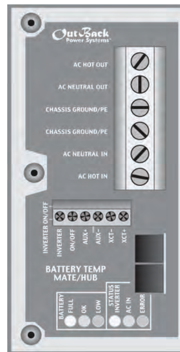
Figure 2 AC Wiring Compartment
